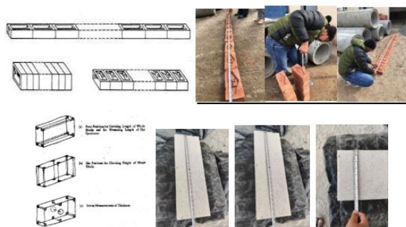
Figure 1: Checking sizes of Red Bricks
