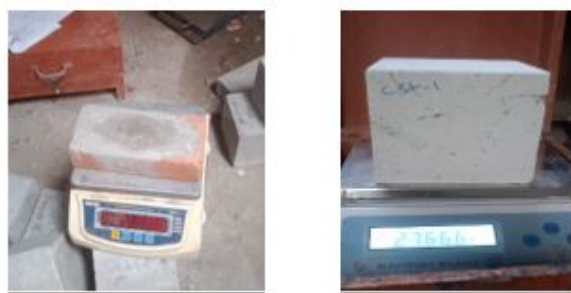
Figure 2: Weighing of samples for Density Calculation
