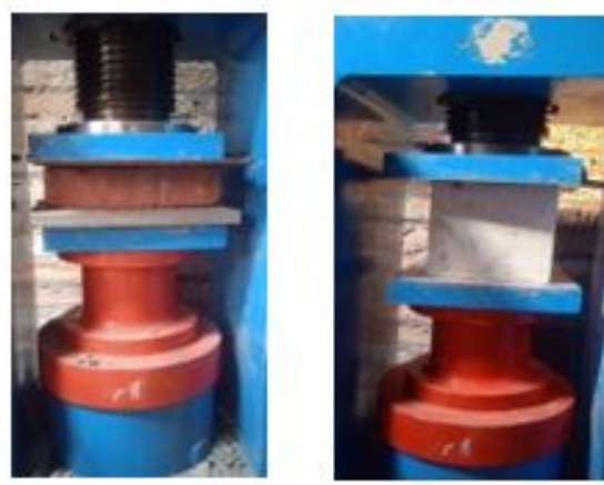
Figure 3: Compressive Strength Test in Compression Testing Machine (CTM)
