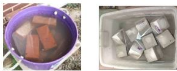
Figure 4: Water Absorption Test
