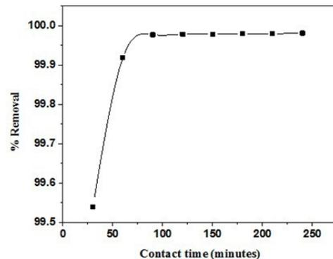
Figure 3: Effect of Contact time on the dye adsorption
