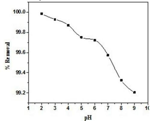
Figure 2: Effect of pH on the dye adsorption
